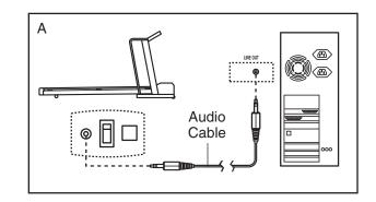
B. Plug one end of the audio cable into the jack on the front of the Incline Trainer near the power cord. Plug the other end of the cable into a 3.5mm Y-adapter (available at electronics stores). Plug the Y-adapter into the PHONES jack on your computer. Plug your headphones or speakers into the other side of the Y-adapter.
